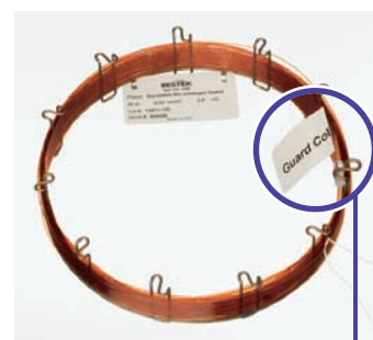
Tag indicates guard column end.
