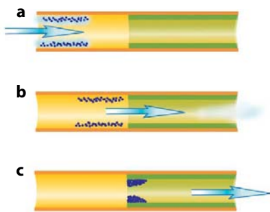
Figure 2 Retention gaps are used to focus components in a tight band at the beginning of the analytical column.
