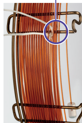
String indicates where the analytical column begins.
