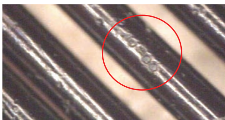
HT fused silica columns, labeled as stable to 430 °C, show pitting and breakdown.
